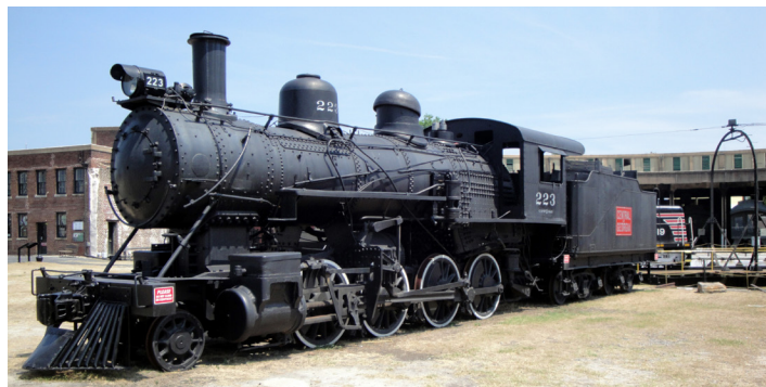
The Central Georgia locomotive no. 223 in front of the roundhouse is a Baldwin C-3 class 2-8-0, built 1907, ended service 1952.
